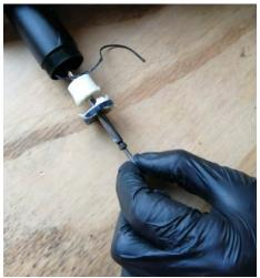
5. Remove the actuator pin from the 6. Using a 5mm allen key remove cartridge - you should be able to pull this out with your fingers.
