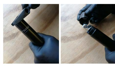
1. Using a 28mm spanner remove the lower cap turning the cap anti-clockwise to undo.
