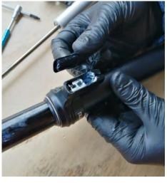
9. Remove the actuator cover (pry this up from the bottom).
