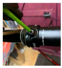
21. Replace the bolt on the collar to 22. The bottom of your post should hold it in place.
