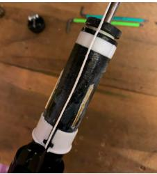
15. With the actuator now positioned, move the top bushing so the string goes through the slot and this should also line up with a slot in the bottom bushing If the string does not line up with bottom bushing, the actuator is in the wrong please so repeat steps 13 and 14 to correctly line everything up.
