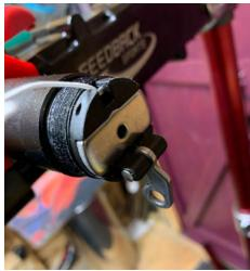
26. The string needs to go over the metal pin on the actuator and then the metal strike plate can be replaced on the actuator.
