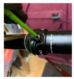
the string through the hole, push the bolt into the actuator then fit washer and nut.
