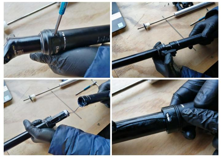
10. On the reverse of the collar undo the grub screw and delicately remove the lower assembly - **ensure you don't lose the guide pin.**
