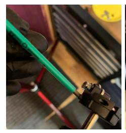
24. Replace the bolt to hold the actuator in place. Be careful not to overtighten. The bolt should not be visible from the opposite side of the actuator.
