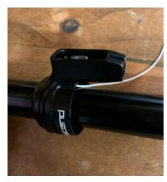
7. Side the collar onto the stanchion, double check the seal is positioned correctly and is not folded over.
