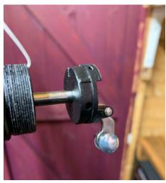
23. Get your actuator and push it onto the bottom of the cartridge. The bolt hole in the actuator should line up with the indent in the cartridge.
