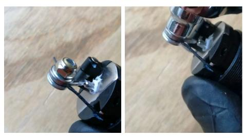
2. Using a 8mm socket carefully undo the nut to release the nylon thread.
