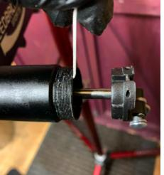
25. Lift the string into the slot inside the post and then push the cartridge / actuator into place. Note that the slot in the actuator needs to go in line with the string.
