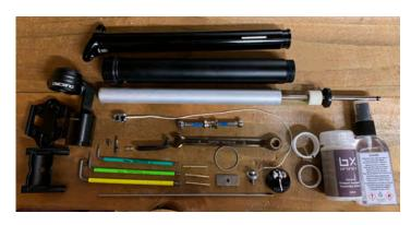
Note – Before you start, **ensure that your cartridge has been compressed halfway**. You can do this by inserting the pin and then pushing down on the cartridge. If the cartridge is at full travel, you will NOT be able to rebuild your seatpost.
