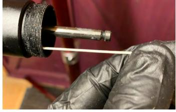
20. Gently pull the string and ensure it moves freely and moves the actuator up, then push the actuator down with your finger to ensure it pulls the string – repeat this step a few times to ensure that the string is moving with no resistance.
