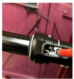
33. You can now push the actuator carefully using a flat head screwdriver to activate it. The post should extend. You can push the actuator again and push the post to ensure it functions as it should If the post is not working as expected, compress halfway, remove the bottom cap and repeat from step 29 onwards.
