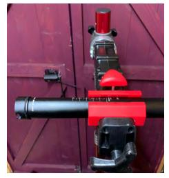
10. Take the bottom part of the seatpost and clamp it horizontally in a workstand with the rear of the post (laser etched markings) facing upwards.
