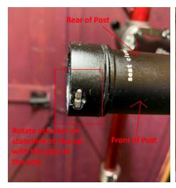
14. Take the stanchion to the seatpost which you have clamped in the workstand. Remember the laser etched part of post is the rear. Rotate the collar on the stanchion to line up the actuator to the area on the post where the string will be inserted.
