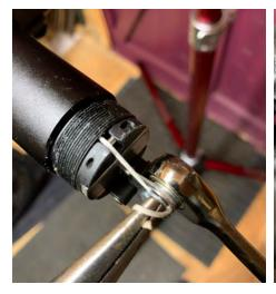
30. Tighten the nut using an 8mm spanner or socket.
