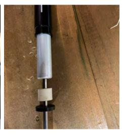
3. Get your cartridge, find the thicker end with the threaded hole and push inside the stanchion then fit the foam spacer and rubber dampner.
