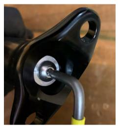
4. Get your bolt and washer then insert into the top of the stanchion and tighten cartridge.
