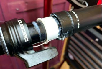
17. Carefully insert the stanchion into the post, if everything has been lined up correctly in the steps above it should slide in easily.
