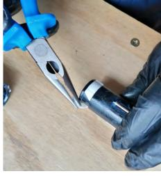
12. Carefully remove the lower bushing.
