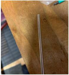
27. Reinsert the long pin Note - The rounded end should be facing outwards.
