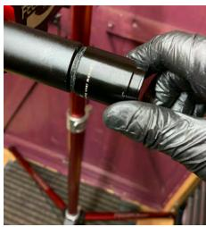
32. Refit the cap on the bottom of the post and tighten with spanner.
