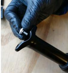
7. Using a 3mm allen key remove the bolt and washer from the head assembly.
