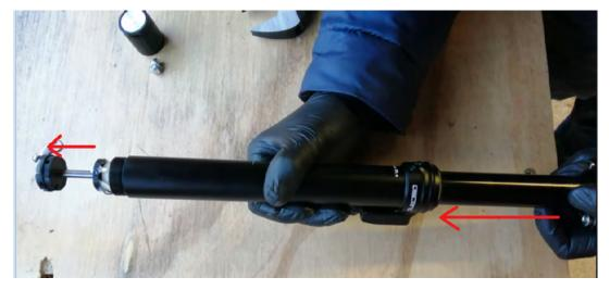
3. Push the shaft of the post to reveal the cartridge.
