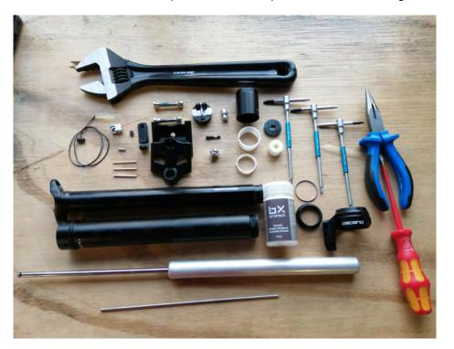
17. Full disassembly is now complete. Inspect the component parts for wear, remove old grease and dirt and exchange worn items for replacements from your maintenance kit. At this stage if required you can also replace your cartridge. Note - these are travel specific and so select based on your existing travel.
