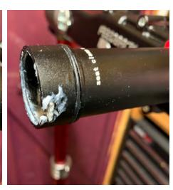
12. Grease cable guide and inner part of post.
