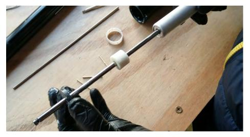
16. Remove the rubber dampener and foam spacer from the cartridge.
